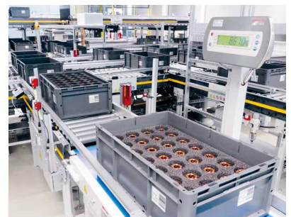
Shuttles supply parts to production just in time.
